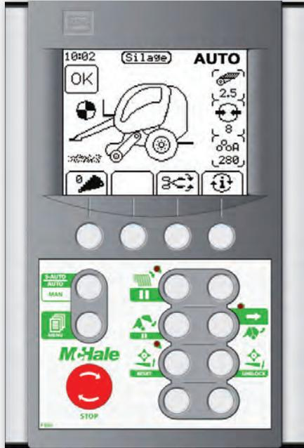
The F5600 is controlled with an Expert Plus Control Box, which features a large graphic display; this allows the operator to monitor the baling process graphically from the control console. It also features;
